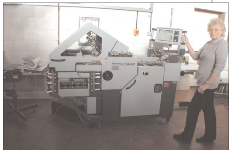
Rosemary Stone, Bindery Technician, with the Horizon AFC-544A automated B2 folding system
