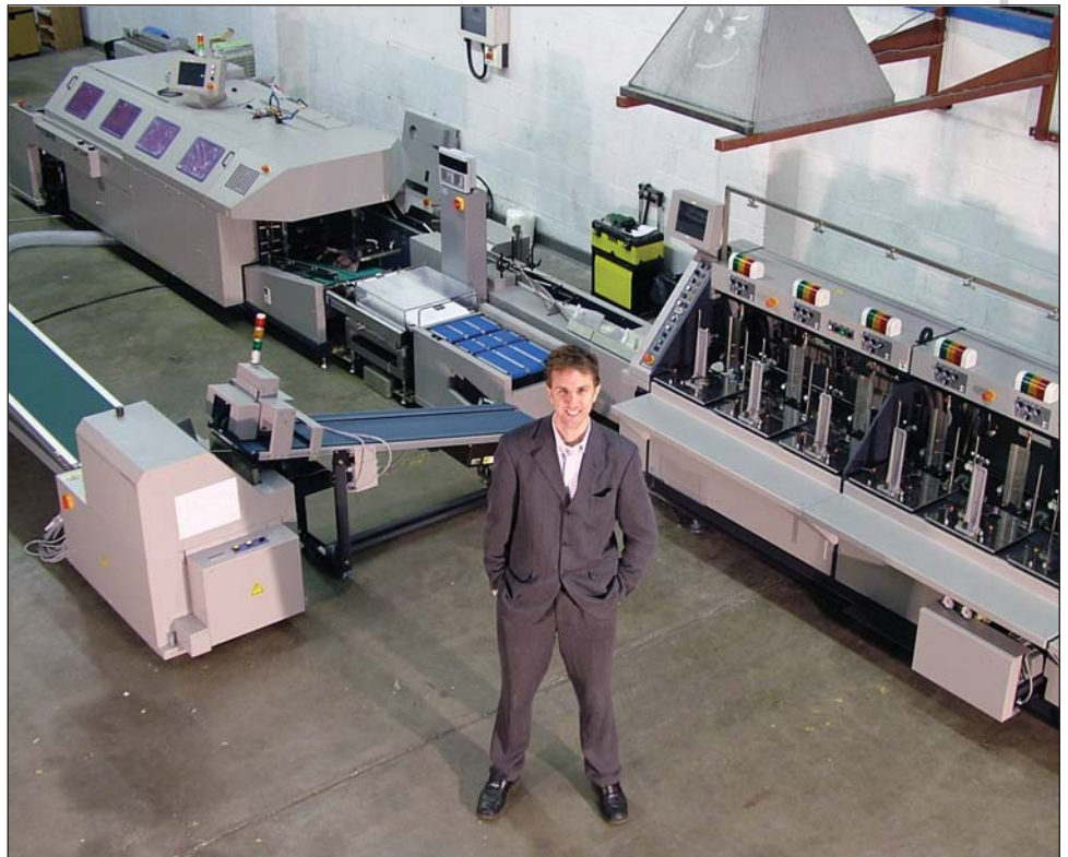
Khromatec Managing Director, Antony Boyes, with the Horizon CABS4000 automated gathering, binding & 3-knife trimming line
